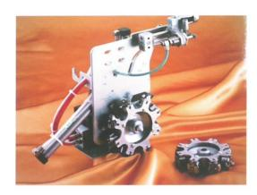
DB-100 for lockstitcher with thread trimmer changes the bobbin automatically by receiving a signal from either the sewing machine or the bobbin checker.
